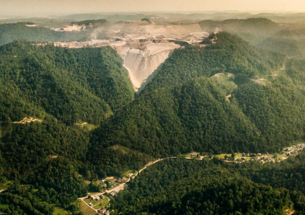
Figures 5.4. (left) and 5.5. (right) Aerial view of a mining site in the hills in the South of West Virginia (US), with a valley filled with mining waste rock. Figure 5.5 shows a close up of the valley fill waste rock dump in Figure 5.4.
